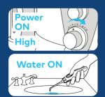
Turn pressure to high, point tip into sink, turn power and water switches ON until water flows. Turn OFF.
