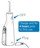
Plug power cord into outlet and connect the charging cord to the unit.
