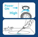
Turn pressure to high, point tip into sink, turn power switch ON until water flows. Turn OFF.
